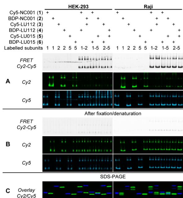
**Figure 3.** Evaluation of six FRET donor/acceptor pairs in HEK-293 and Raji lysates. (A) Native-PAGE analysis. (B) Native-PAGE analysis after gel fixation. (C) SDS-PAGE analysis to verify correct labeling. Gels were imaged using Cy2, Cy5 or Cy2-Cy5 settings, see Figure S1. See Table S2 for calculated FRET efficiencies.
